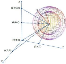
**Figure 1.** The five dipoles' locations utilized for the formulation of the inverse scattering algorithm determining the center's coordinates and the layers radii of a 2-layered sphere with a PEC core.
