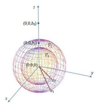
**Figure 2.** The two dipoles' locations utilized for the formulation of the inverse scattering algorithm determining the material parameters of a 2-layered sphere with a dielectric core.
