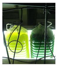
Figure 1. Cultivation of the cyanobacterium *A. platensis* in photobioreactors of 10 L volume (left: carbohydrate-enriched biomass, right: conventional composition biomass).
