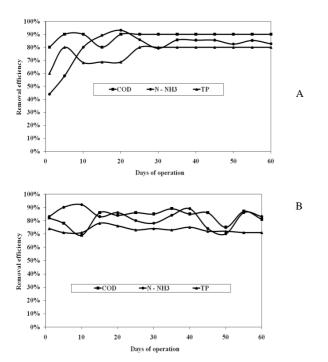
**Figure 3.** Removal efficiencies of COD, ammonia – nitrogen (N-NH3) and total phosphorus (TP) with time are shown as average values for the reactors A) without (R) and B) with (RB) the presence of PVA biofilms.
