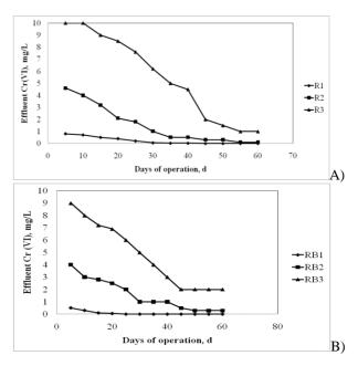
**Figure 4.** Effluent Cr(VI) concentrations for A) activated sludge reactors (R) and B) biofilm reactors (RB)
