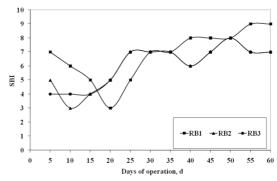
**Figure 10.** SBI values as a function of operation time for biofilm reactors (RB)
