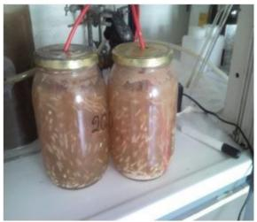
Figure 1. Reactors supplied with PVA beads
