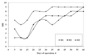
**Figure 9.** SBI values as a function of operation time for activated sludge reactors.
