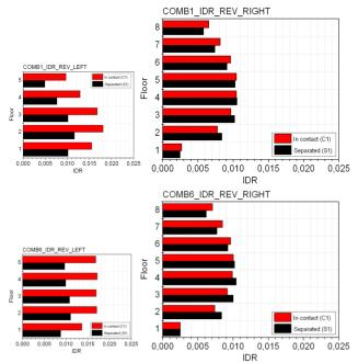
Figure 7. Max. interstorey drifts: BC#1 - BC#6 and REV earthquakes.
