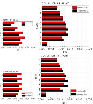
Figure 8. Max. interstorey drifts: BC#1 - BC#6 and S-S earthquakes.
