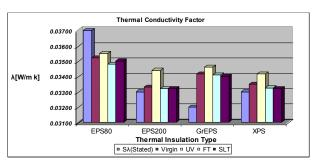
Figure 4. Thermal Conductivity " $\lambda$ " Graph
