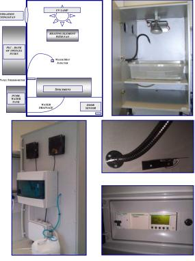
Figure 1. - Constructed Chamber/Apparatus for UV Stress Test
